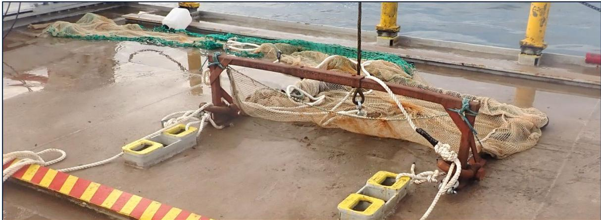
Figure 8 Scientific 2m Beam Trawl.
